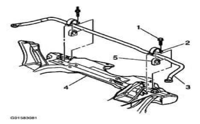
Fig. 7: Stabilizer Shaft Courtesy of GENERAL MOTORS CORP.
