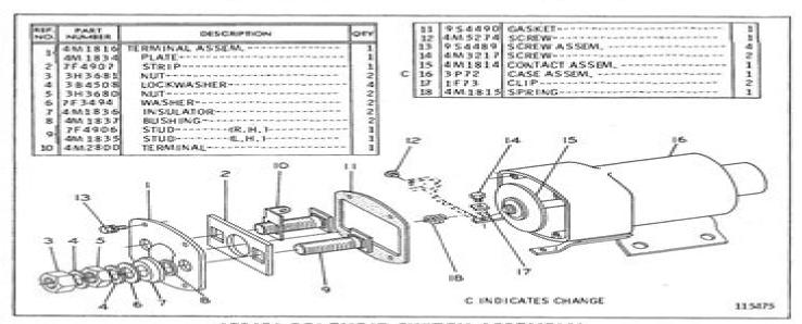
1P9181 SOLENOID SWITCH ASSEMBLY Part of 4N3182 Electric Starting Motor Group shown on Page 32
