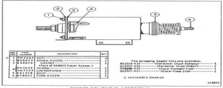
9S7976 SOLENOID ASSEMBLY Part of 2P6162 Electric Starting Motor Group shown on Page 30
