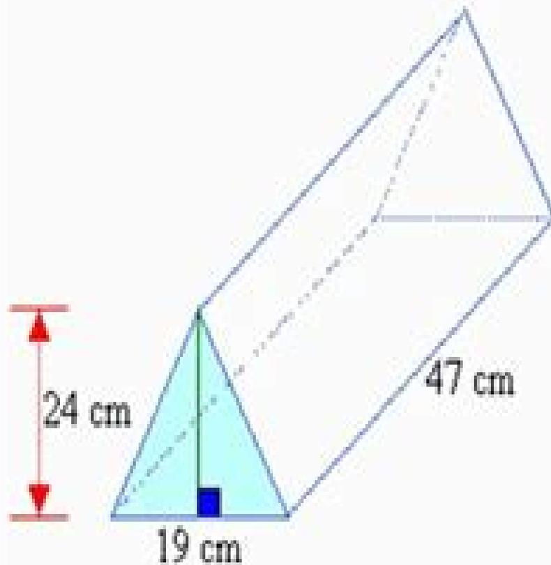
$$\begin{aligned}V &= \frac{B \times H \times L}{2} \\&= \frac{19 \text{ cm} \times 24 \text{ cm} \times 47 \text{ cm}}{2} \\&= \frac{21432 \text{ cm}^3}{2} \\&= 10716 \text{ cm}^3\end{aligned}$$
