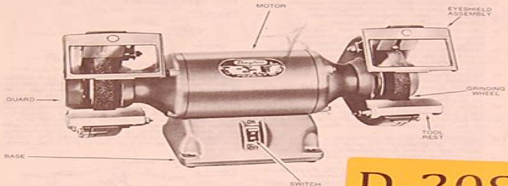
Figure 1 — Dayton Bench Grinder Nomenclature
