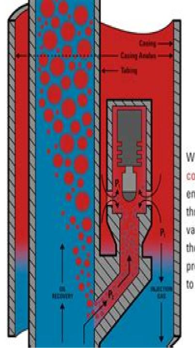
When the compressed gas enters the tubing through the gas lift valve, the energy of the expanding gas propels the oil closer to the surface.
