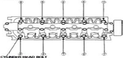
CYLINDER HEAD BOLT 10 x 1.25 mm 73 N·m (7.3 kg·m, 53 lb-ft)
