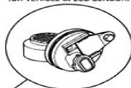
AUTOMATIC TRANSMISSION OUTPUT SPEED SENSOR (OR VEHICLE SPEED SENSOR)
