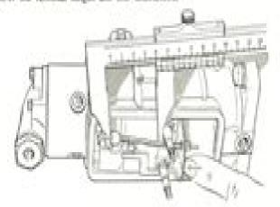
Fig. 7 Measurement of governor link length
