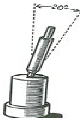
Illust. 66. Checking wear and alignment of the valve pintle.
