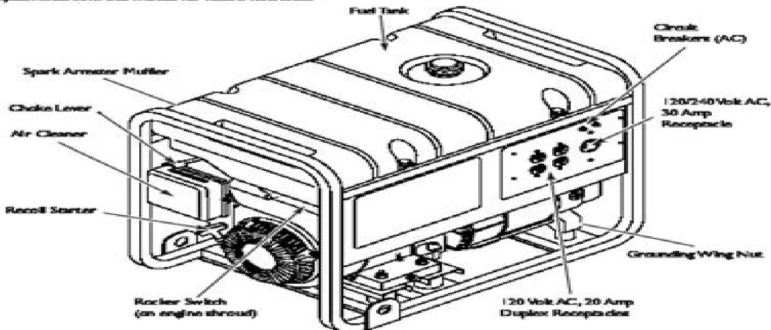
**120 Volt AC, 20 Amp, Duplex Receptacles** — May be used to supply electrical power for the operation of 120 Volt AC, 20 Amp, single phase, 60 Hz electrical lighting, appliances, tool and motor loads.
