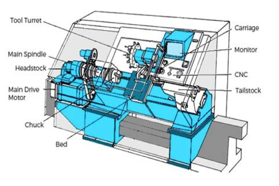
Diag. Main parts of a CNC lathe machine
