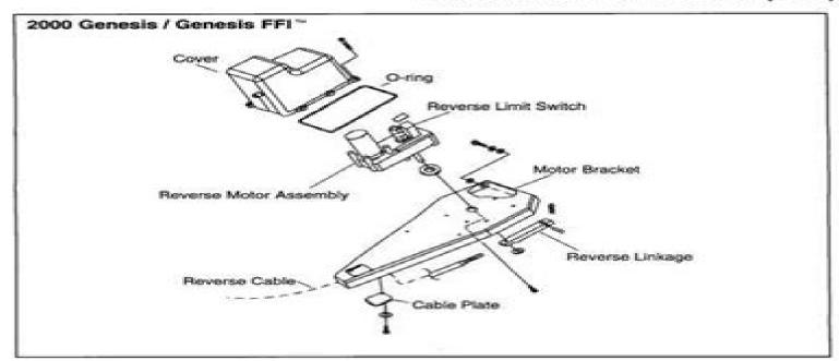
The Genesis watercraft feature an electric reverse gate system designed to make changing direction of travel easier for the operator. A simulated "neutral" gear is possible by positioning the reverse gate half way down. Engine power is limited for safety when the reverse gate is not in the full up or forward position.
