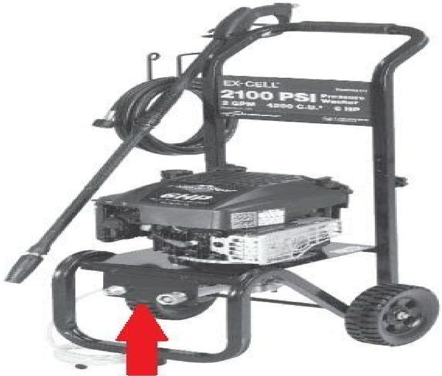
**This is where the frame must be altered in order to use the new style Inlet/Outlet tubes**
