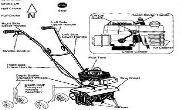
Throttile Control — Controls the engine speed and the tine rotation. This cultivator is equipped with a centrifugal clutch that engages the tine drive system when the engine speed is increased.
