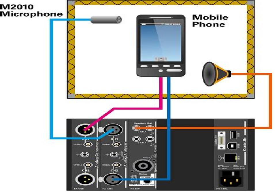
FX100 Audio Analyzer with FX-SIP
