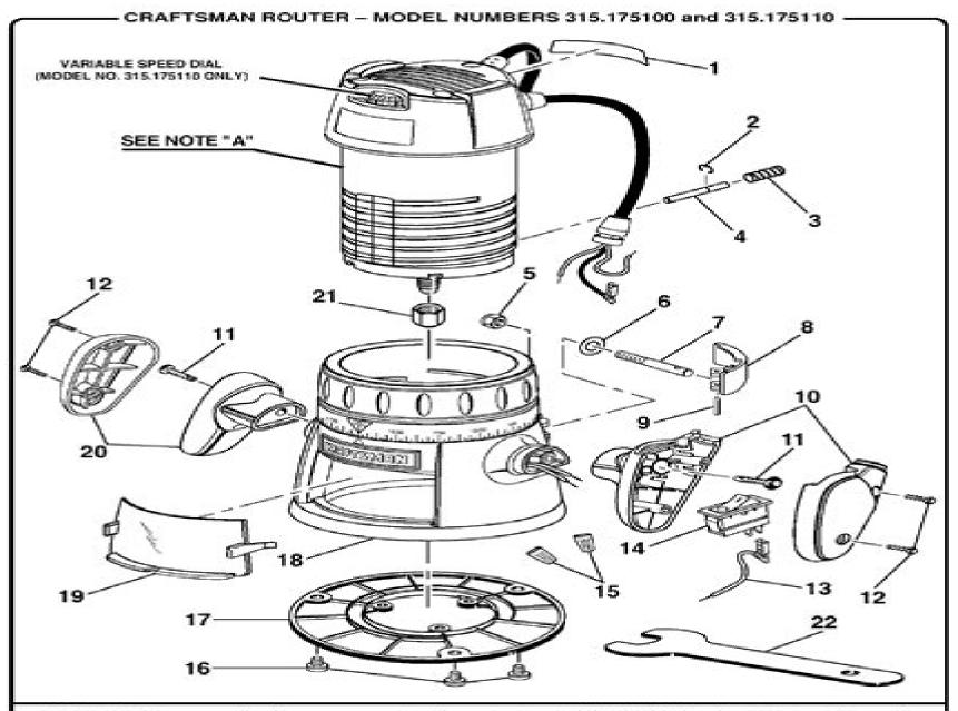
NOTE: "A" - The assembly shown represents an important part of the Double Insulated System. To avoid the possibility of alteration or damage to the System, service should be performed by your nearest Sears Repair Center. Contact your nearest Sears Retail Store for Service Center information.
