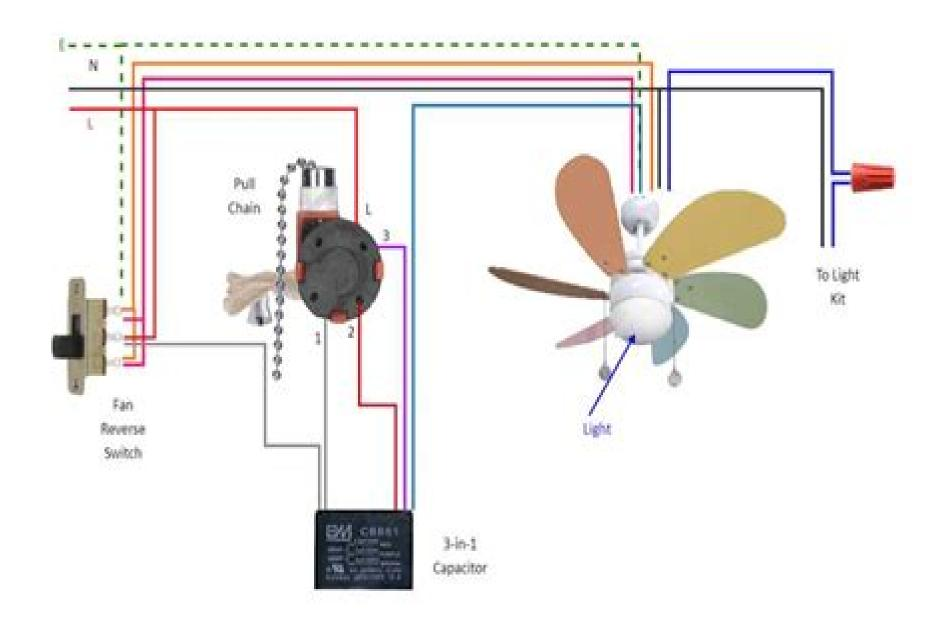
3 in 1 Celing Fan Capaictor Wiring with Pull Chain, light Kit & Reverse Switch
