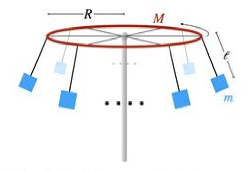
The support ring (red) and chairs (blue) are massive, with masses as shown, while all other structures are massless. Two relevant lengths are noted. There are N chairs, each of which can swing axially—i.e., it can only swing about an axis tangent to the support ring at its point of contact. The support ring is free to rotate about the central pole.
