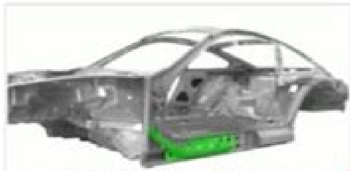
Isolation position of lower side member reinforcement
