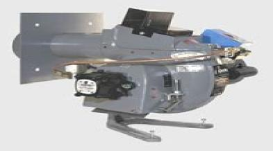
"CRD" burners feature a combustion head incorporating a new design concept which provides a means to control the air pattern to match the nozzle requirements. The aero-dynamics for optimum combustion are easily adjusted for any nozzle size without changing the air-handling hardware. The flame front is initiated inside the air tube so that no erratic recirculating gasses from the main chamber area can quench the flame at the retention ring.
