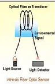
OF experiences geometrical (size, shape) and optical (refractive index, mode conversion) changes applied external perturbations.
