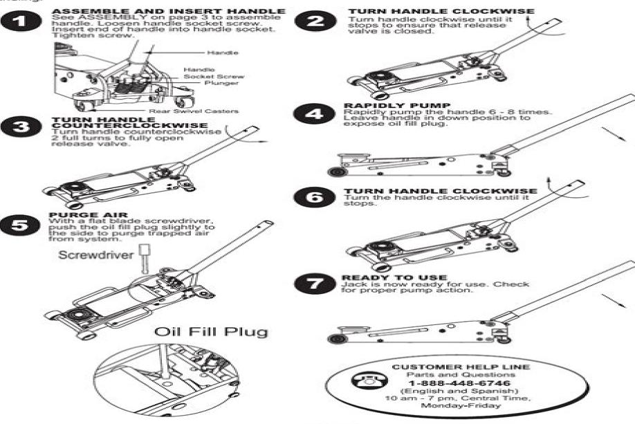
NOTE: Repeat this Air Purge Procedure whenever the jack displays reduced lifting performance.
