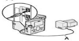
Connect the machine and your computer with a USB cable (A).
