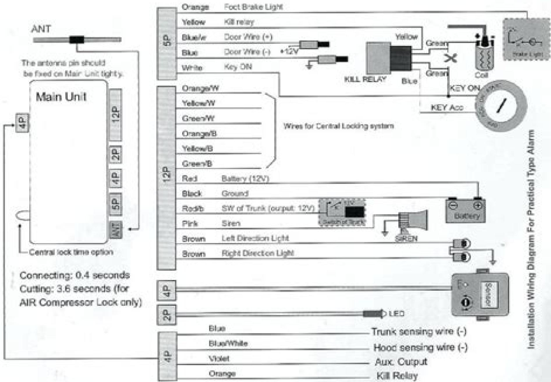
Installation Wiring Diagram For Practical Type Alarm
