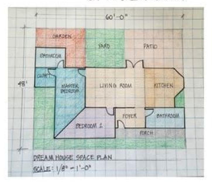
You will develop a space plan on grid paper at the scale of 1/8° = 1 foot
