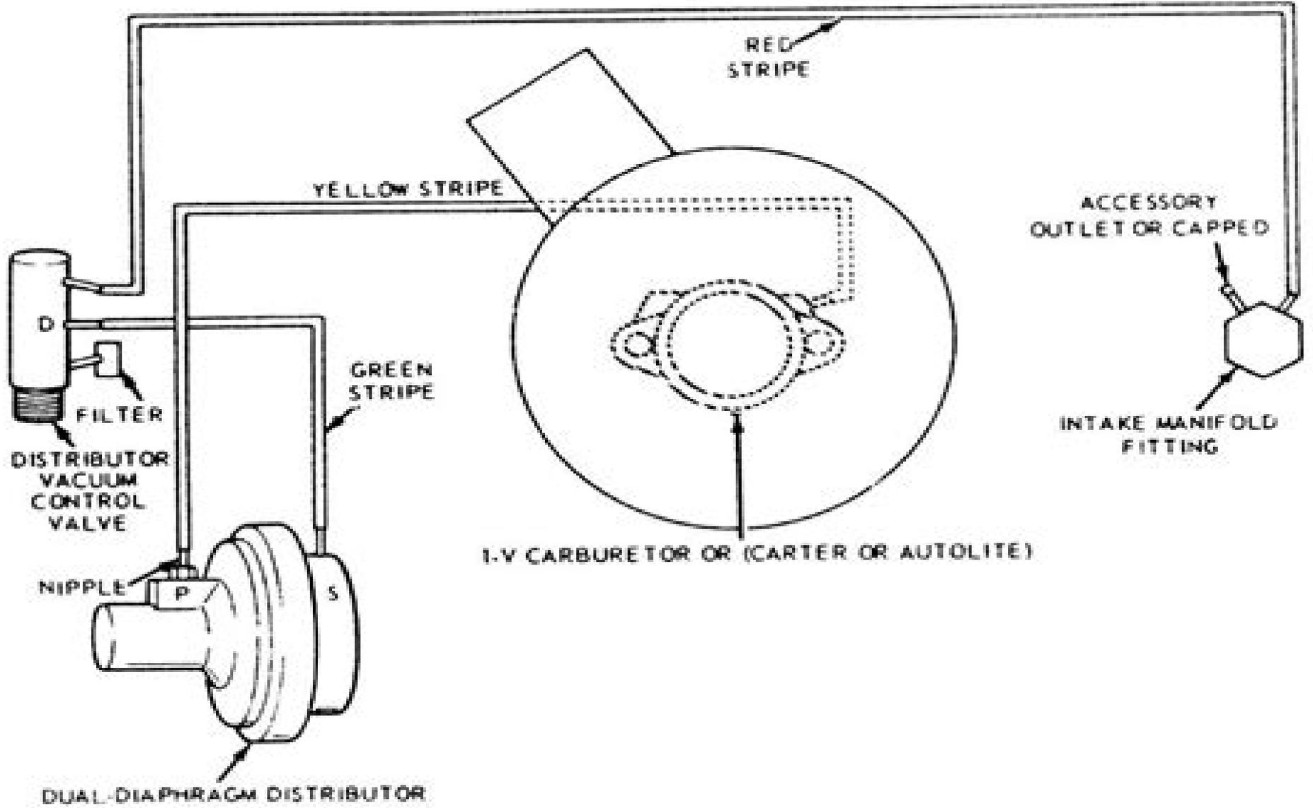
**1968 Ford 170, 200 1-bbl., IMCO with automatic transmission without air conditioning in Cougar, Fairlane, Falcon, Montego and Mustang**
