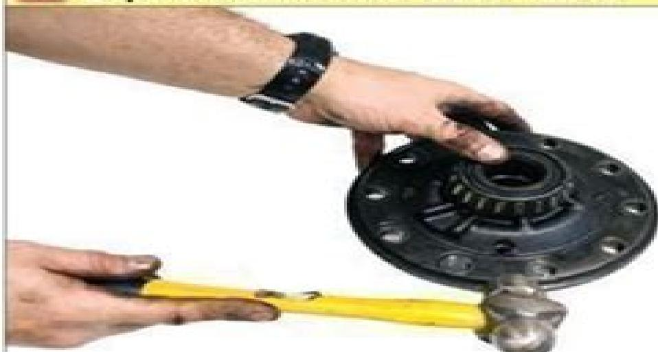
The differential case halves should come apart easily. Since this is an open differential, there are no other fasteners or clutch pack preload to overcome to separate them.
