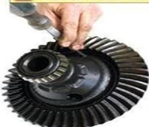
Use the appropriate-size punch to drive out the roll pin. You can use a long, 1/4-inch punch. You can remove the pin now or wait until the ring is removed. The order doesn't matter.
