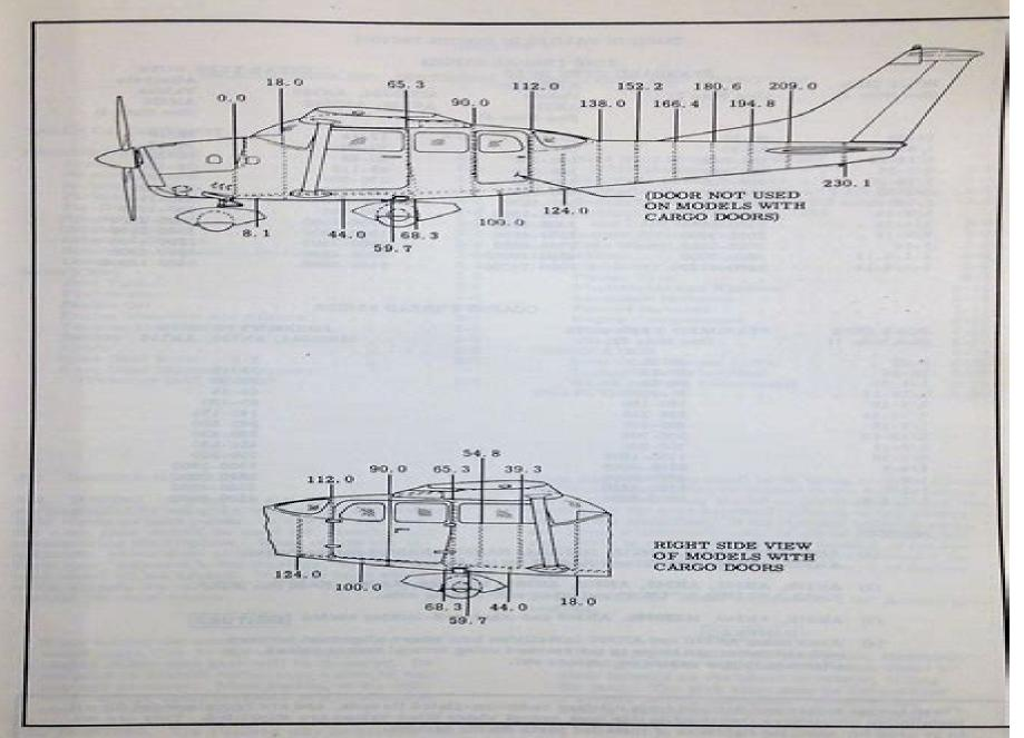
Figure 1-3. Fuselage Reference Stations (Model 206 Series)
