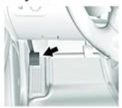
Set the parking brake by holding the regular brake pedal down, then pushing down the parking brake pedal.
