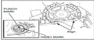
Make sure the piston is at TDC (Top Dead Center) on the compression stroke.
