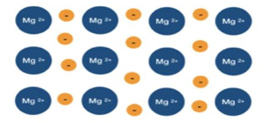
Figure 1. Magnesium is a metal which has a giant structure. This figure represents an example of metallic bonding between magnesium ions and the delocalised electrons. Each Mg atom loses 2 electrons to form a full outer shell, so the Mg ions have a charge of 2+.
