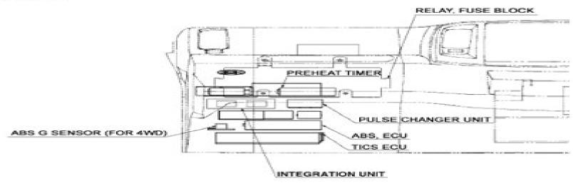
The figure shows RHD VEHICLE, LHD VEHICLE's figure is symmetrical.
