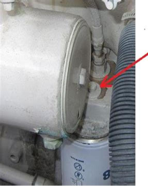
Best Oil Pressure test point on any Cummins B
