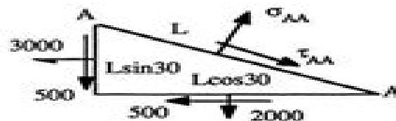
$$\begin{aligned}\sum F_{n,AA} &= 2500L - (\sigma_{xy} \cos 30^\circ + 2000 \sin 30^\circ)L \sin 30^\circ \\ &\quad - (\sigma_{xy} \sin 30^\circ + 3000 \cos 30^\circ)L \cos 30^\circ = 0\end{aligned}$$
