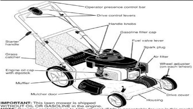
NOTE: Gasoline containing up to 10% ethanol (E10) is acceptable for use in this machine. The use of any gasoline exceeding 10% ethanol (E10) will void the product warranty.
