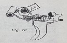
SECONDARY SEAR ENGAGING "BURST" NOTCH IN HAMMER
