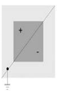
Square sheet with outer conductivity  $\sigma$ =1 and inner conductivity  $\sigma$ =0.5.
