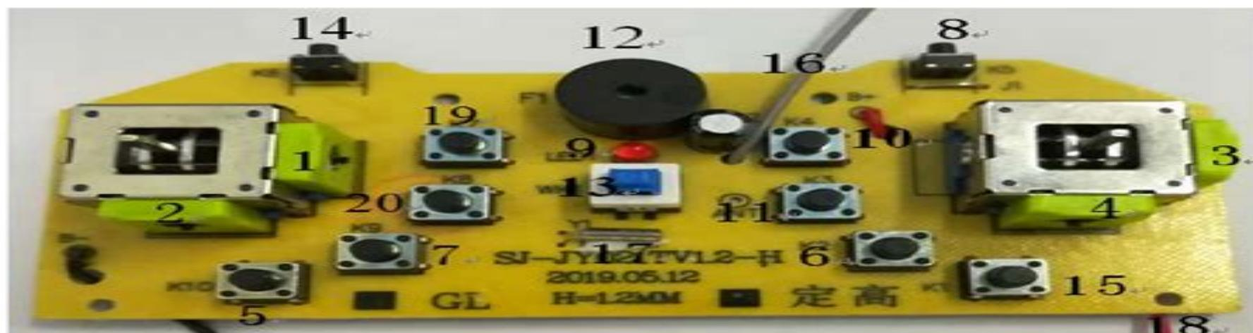
1 and 2: Throttle potential controller and left and right steering potential controller
