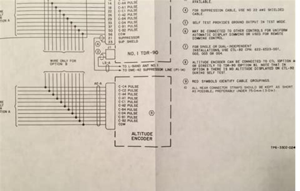
TDR-90 Interconnect Woring Diagram, Pro Line II, CSDB, Single Installation Figure 2-7
