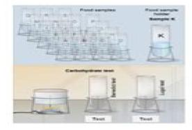
The Benedict test is a test for monosaccharides; simple sugars like glucose or fructose (fruit sugar). In contact with monosaccharides, the Benedict solution turns from blue to green to orange.
