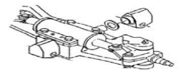
If silent blocks have been removed from axle, install new silent block assemblies and thrust washers (or spacers, as applicable, depending on steer axle model). See Page 9.7-2 (see Page 9.5-4 for Type 2 axle).
