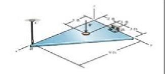
"5-76. The member is supported by a pin at A and a cable BC. If the load at D is 300 lb, determine the  $a_i$   $y_i$  zcomponents of reaction at the pin A and the tension in cabbe B.C.
