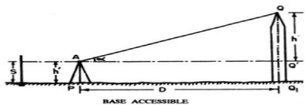
h = D tan α Height of the object = s + h R.L. of top of the object = R. L. of B.M. + s + h
