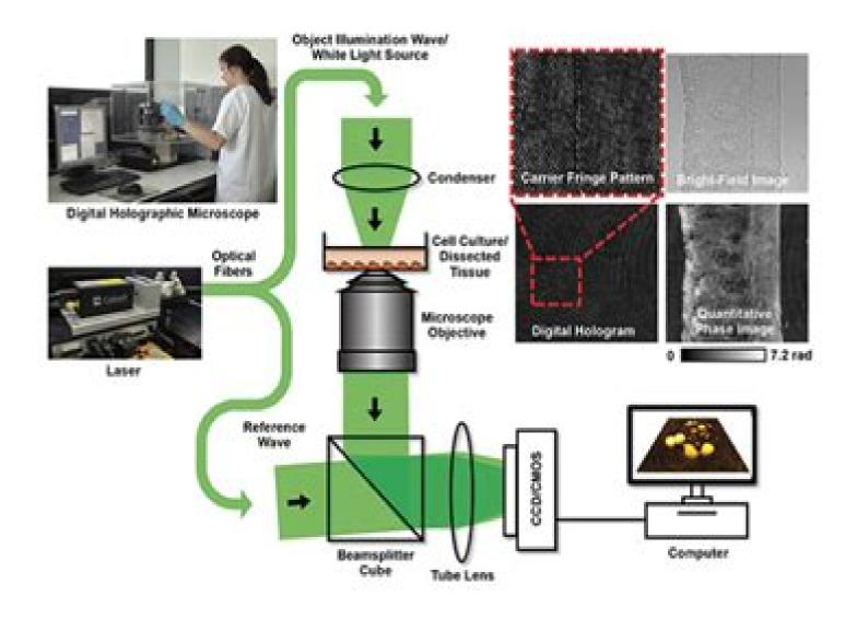
Figure 1. The concept of laser-based inverted off-axis DHM in transmission configuration for correlated label-free bright-field and quantitative phase imaging of dissected tissues (upper right) and living cell cultures in the environment of a biomedical laboratory. Adapted with permission from References 3 and 4.
