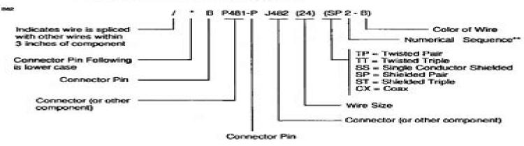
\*\* A numerical sequence for each type of wire (SP1, SP2, SP3, ST1, ST2, ST3) on a wire diagram page may be used to identify wires within a shield or twisted group when they are not drawn adjacent and enclosed by a twisted or shield symbol. Example: SP2-B and SP2-W are the two wires within a shield.
