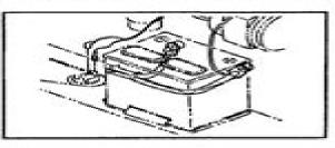
7. Check battery for damage and cleanliness of terminals. Remove the boot covers to expose terminal connections. Clean battery terminals and cable connections if they are dirty and corroded. Check battery terminal cable connections for tightness. Replace boots over terminals after inspection. If necessary, wash battery with a mild solution of baking soda and water. First, make sure that cell vent caps are tight to ensure that soda solution does not contaminate battery electrolyte.
