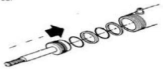
Coat the gland with a light coat of oil. Carefully slide the gland over rod and into the cylinder bore making sure the seal is not damaged in the process.
