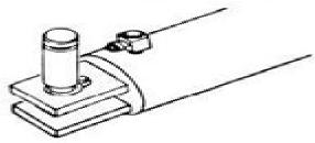
Position the opposite end in the upright yoke and insert the tilt pin into this yoke.
