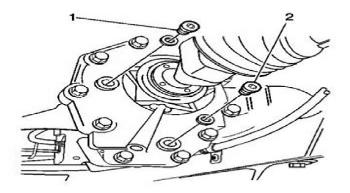
Fig. 2: View Of Differential Drain Plug Courtesy of GENERAL MOTORS CORP.
