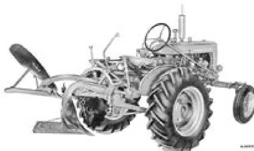
No. 151 Moldboard Plow with notched bottom and combination jointer.
