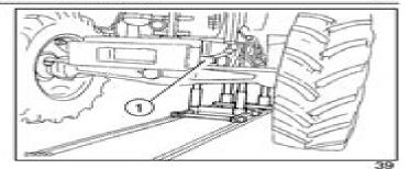
Insert a wooden block between the stands and the tractor.
