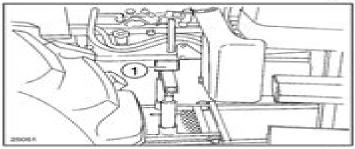
Place a fixed stand (1) underneath the drawbar support and apply the handbrake.
